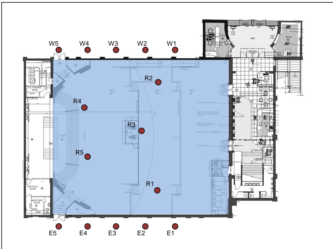
Figure 3 – Microphone positions for eastern façade, western façade and roof void
